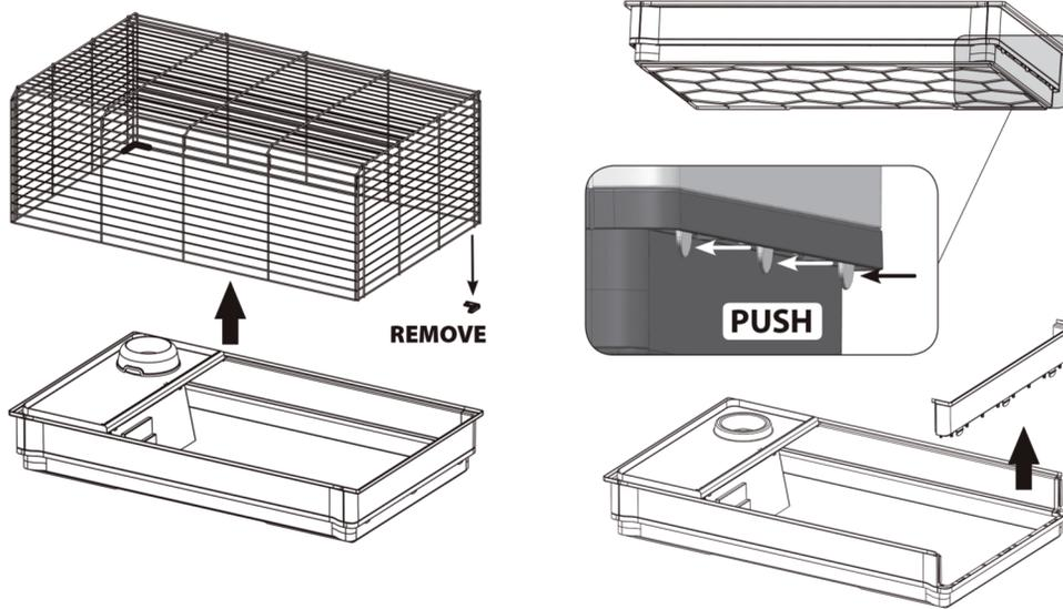
6. Assemble the 158HEX bottom tray. Connect the two plastic sides (B) to the plastic bottom (A) as shown. Make sure the tabs on each side of the bottom slide into the grooves of the sides.
