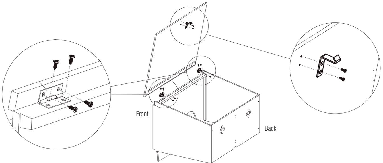
NOTE: When assembled correctly, the lid will lie flush on the top of the hutch with no gaps along the sides, and the end of the "S hook" will be exposed on the outside, below the back lip of the lid.
