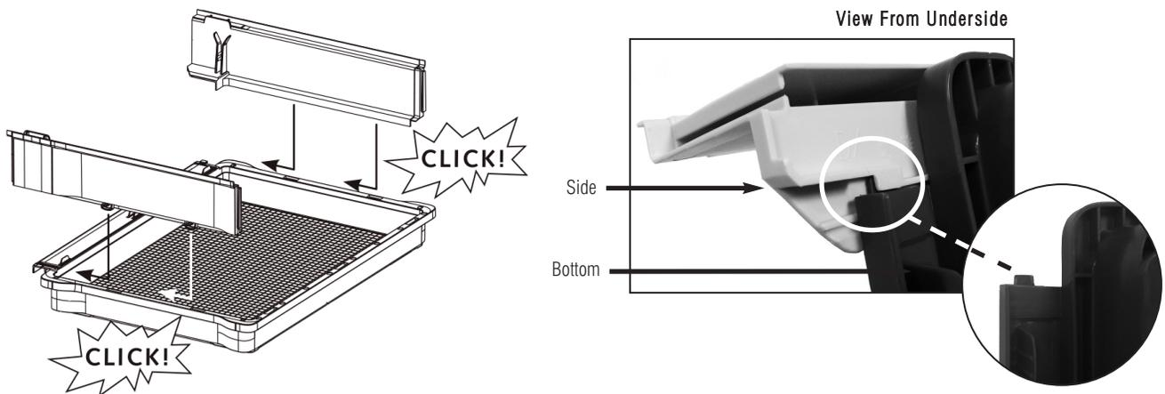
7. Attach the assembled extension bottom to the plastic bottom of the 158 base unit. Attach the end that was removed from the 158 base unit in Step 5 to the end of the extension.
