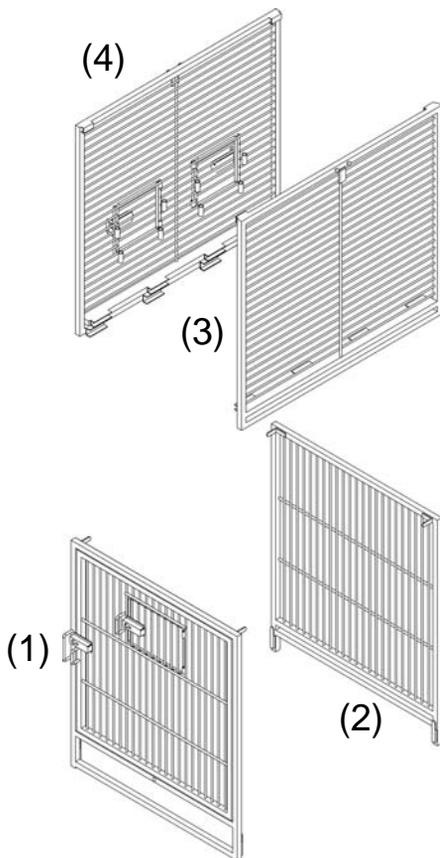
1. Take the FRONT PANEL, BACK PANEL, AND both SIDE PANELS and arrange them as shown in the drawing to the left. On the bottom, interior of both the FRONT and BACK PANELS there are two small prongs jutting up. Take the FRONT PANEL and either of the two SIDE PANELS and insert the hollow square tube at the bottom of the SIDE PANEL onto the top of one of the prongs.
