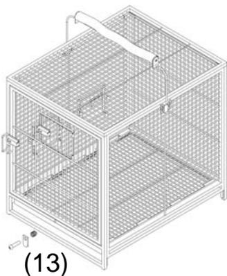
5. After the four primary panels are together, take the TOP GRATE with its four pairs of “feet” facing downward, and fit the four pairs of feet into the square tubes at the top of the four PANELS.
