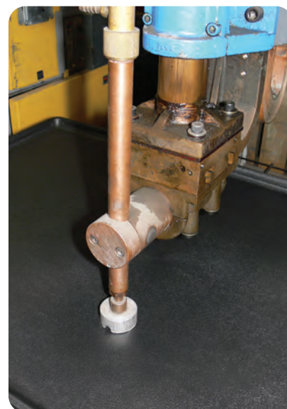
A Continuous Impact Test is used to test the durability of our plastic crate pans.
