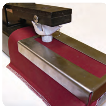
A Crockmeter is used for testing the transference of color from the surface of one material to another by either wet or dry rubbing.
