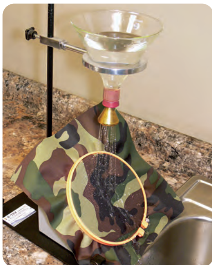
The Water Repellency Test measures the resistance of fabrics to wetting.
