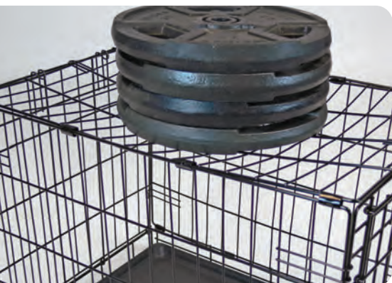
A Static Load Test is used to test the durability of a crate.
