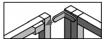
**8** Locate the Bottom Grid (G) and the Bottom Pan (H.) The Pan can be inserted in two different positions, depending on the use of the Bottom Grid.
