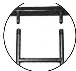
**17** Locate the Ladders and slide them onto the angled posts on the Perch.
