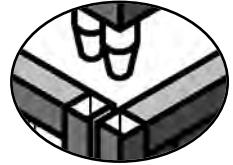
**Bottom Grid will be used:** Slide the Bottom Grid in the rails just below the front door. Slide the Bottom Pan immediately under the Bottom Grid.
