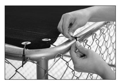
After the corners have been attached, loosely affix a Long Plastic Tie at each grommet on the Sunscreen around the perimeter. Starting at one corner, pull the tie a bit tighter. Work your way around to each corner, pulling the ties tighter and tighter until they are all snug. Now work your way around the kennel, pulling the remaining ties up as you go.
