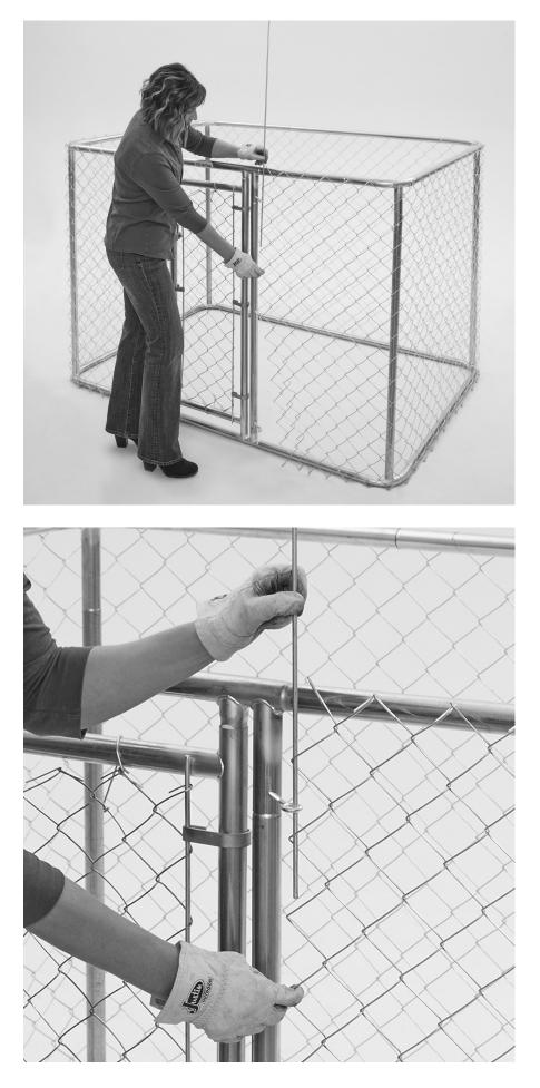
**18.** Facing the Kennel door, go to the top left Eyebolt. Push the "eye" firmly against the Gate Frame. Tighten the Nut past the scored area of the bolt's threads. Move down to the next Eyebolt and repeat. Pulling the Tension Rod against the Gate Frame as you go, proceed around the Gate Frame until all six Eyebolts have been tightened. This step will tighten the fit of the Chain-Link Fence around the frame.
