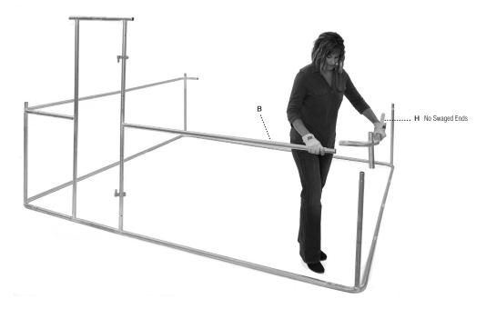
**7.** Place the final Bent Middle Rail (H) with one swaged end and one non-swaged end on the last Vertical Corner Post. Connect the two Bent Middle Rails on the side.
