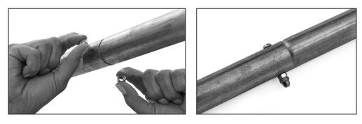
**3.** Push the swaged ends of each rail into the non-swaged ends of each adjacent rail, making sure all pieces are pushed in completely and put together firmly.
