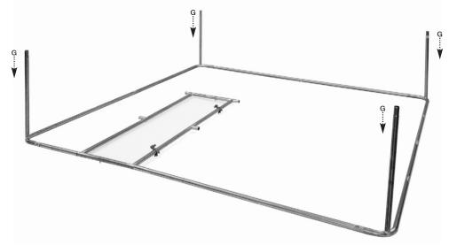
**5.** To assemble the middle rail, start at the corner closest to the Gate Frame. Swing the Gate Frame into the upright position. Use a Short Filler Rail (E) to connect the Gate Frame to a Bent Middle Rail (H) with NO swaged ends. Secure the long peg of the Bent Middle Rail on the Vertical Corner Post.
