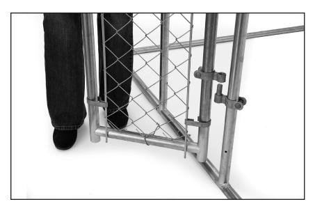
**13.** Align the top knuckle with the top pin on the door. Adjust the top knuckle as needed, making sure that when the door swings, the bottom of the door will clear the bottom rail on the ground and that the top of the door will clear the top rail. Slide the knuckle over the pin and loosely tighten the knuckle. Check once more to ensure the knuckle placement will allow the door to swing within the opening. Then, use a wrench or socket wrench to tighten the bolts on the door's knuckles.
