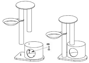
**5.** Place the Bolstered Pillow (H) on the Platform and secure with the drawstring. With a Phillips screwdriver and the Tiny Screws (P), attach the Dangle Ball (Q) to the post.
