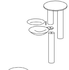
**4.** Align the assembled Posts with the holes in the Base and the top of the Cubby. Place a Washer (K) on the Dome Head Screw (O) and attach the shorter post to the top of the Cubby. Tighten with the Allen Wrench (R). Secure the longer post to the Base using the screw in place from Step 1. Tighten with the Allen Wrench.
