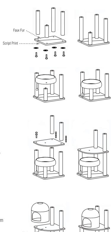
5. Place the Upper Platform (J) on the two Medium Sisal-Wrapped Tubes (G). On the Script Print fabric side, insert a Dual-Thread Screw (O) through the platform and into the Medium Sisal-Wrapped Tube (G). Use a flathead screwdriver to tighten. Attach a Short Sisal-Wrapped Tube (C) to top of the Upper Platform, over the Dual-Thread Screw. Turn clockwise to tighten.
