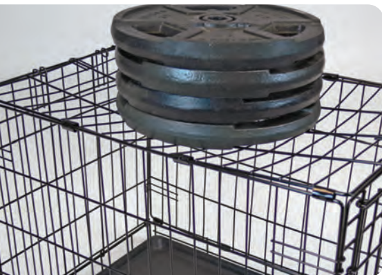
A Static Load Test is used to test the durability of a crate.
