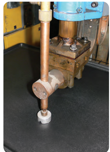
A Continuous Impact Test is used to test the durability of our plastic crate pans.
