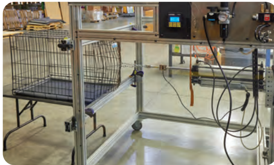
The pull-tester allows us to test the strength of the wire, latches, and overall construction of our containment products.
