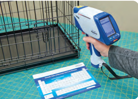
The XRF PMI gun analyzes the chemical composition of our metal products and verifies that our quality and safety standards are consistently met.
