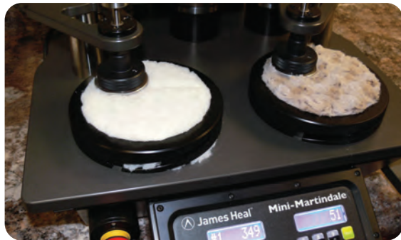
A Martindale Abrasion Tester is used to check the abrasion and pilling resistance of fabric. Fine grit sandpaper is used to replicate the pad of a dog's paw.
