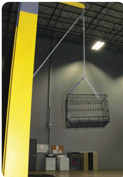
A Drop Test is used to test overall functionality of the crate and its components after 3 drops from three feet.
