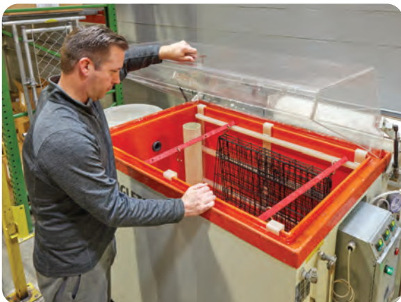
The corrosion test chamber evaluates the rust-resistance of coated wire, hardware, and other metal components.
