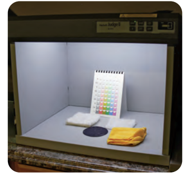
A Light Box allows us to look at the results of our tests under different types of light, including daylight, fluorescent and incandescent light.
