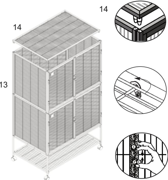
**13.** Attach the Side Panels by inserting the pegs into the holes between the Door and Back Panels. Be sure the cut-outs on the bottom go around the protruding wires of the Bottom Floor Panel Grid. Insert the protruding tabs at the top of the panels into the protruding openings in the Door and Back Panels to lock the panels together.
