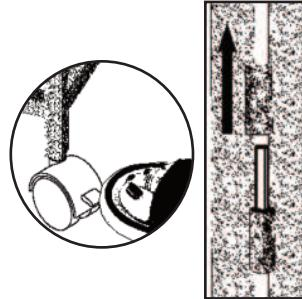
**Locking Casters** The front casters can be locked to prevent any unwanted movement of the cage.
