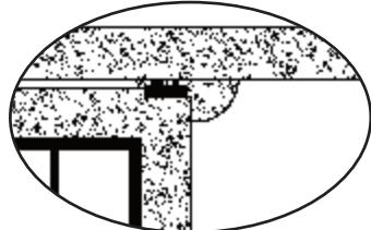
**No-Doubt Door Latches** The squeeze point latches are easy for humans to operate, but impossible for pets! When closing and latching the doors, be sure the spring-loaded rods have been fully inserted into the holes in the door frame. To help make this easier, there is a plate at the top and the bottom in the middle of the door frame. This will line up the door so the rod will fit right into the holes.
