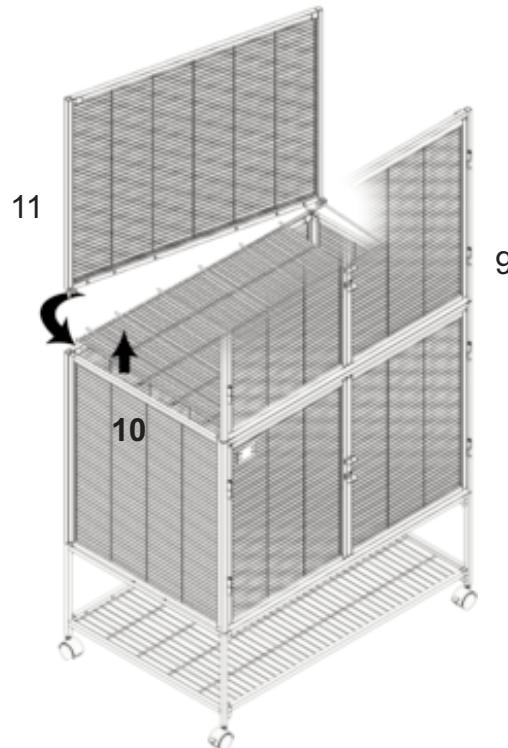
**10.** Locate the Middle Floor Panel Grid (G) and insert the protruding wires into the corresponding holes of the Door Panel. Orientate the panel so the opening is either in the back-right or front left of the cage.
